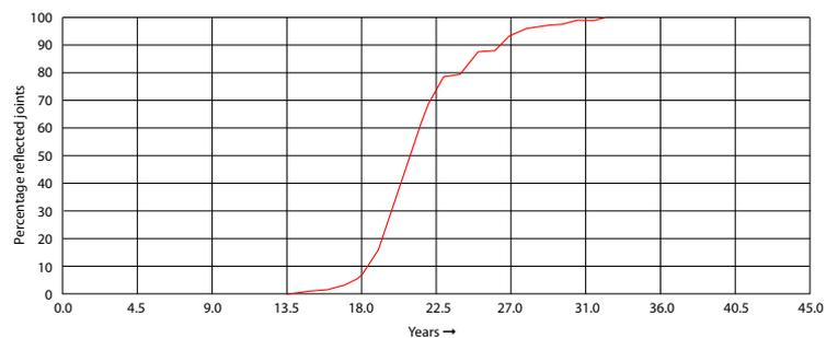
Diagram 2 – Expected % reflective cracking performance versus years in service
