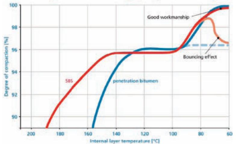
Good workmanship: When continuing compaction till 60 °C (internal layer temperature)
