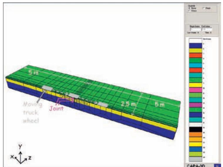
Diagram 3 – Finite element analysis mesh used for the A45.
