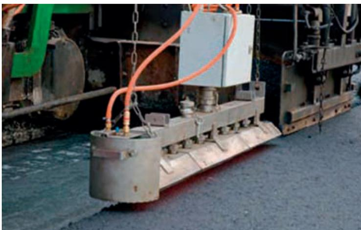
Picture 5 – Material Edge, Ecos seam Joint Heater in use.
