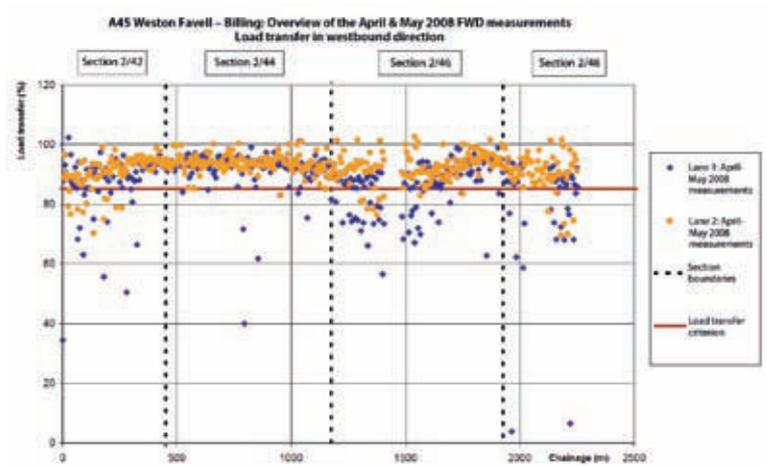
Diagram 1 – FWD measurements, load transfer west bound
